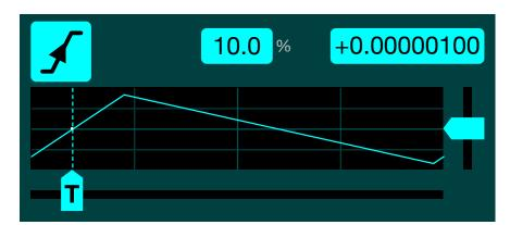
An oscilloscope's trigger system is one of its **most important** functions. Triggering is what enables the scope to display repetitive waveforms in a steady fashion - allowing us to see our audio in a clear and meaningful way. The trigger makes repetitive waveforms appear static by repeatedly displaying similar portions of the input signal. A trigger system also lets you capture single-shot waveforms.
