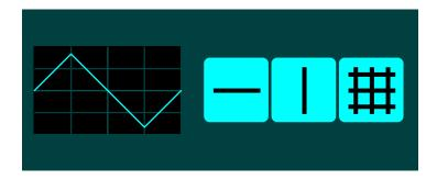
auSCOPE X lets you turn on or turn off the vertical and horizontal center reference lines independently. You also have control over whether to show or hide the grid.
