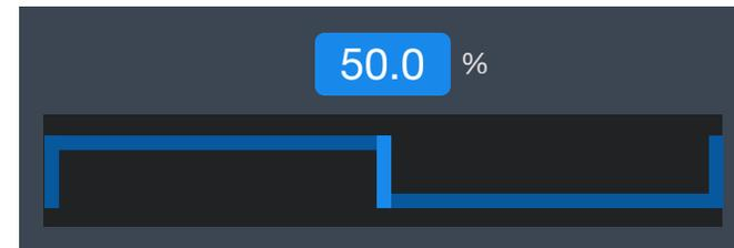
Setting the Rectangle to 50.0% Duty Cycle gives you the classical Square Wave. Setting the Triangle Duty Cycle to the low extreme (1.0%) approximates a falling Sawtooth while the high extreme (99.0%) gets close to a rising Sawtooth.
