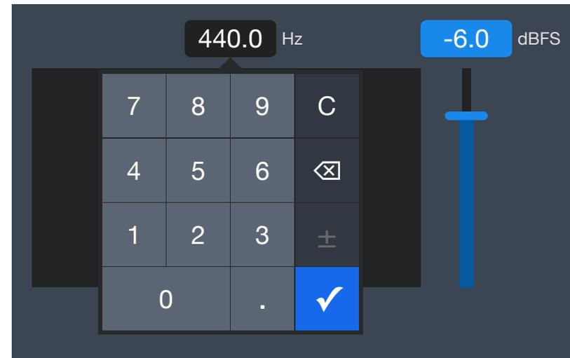
Lastly, all of the numeric parameter readouts are actually buttons. Tapping on one will bring up a convenient number keypad so you can directly enter in an *exact* value. And for
