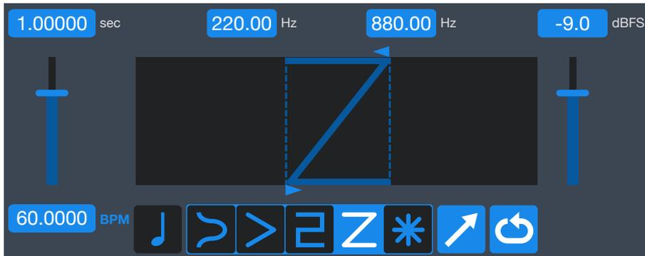
Next, you'll find an additional control for setting the Sweep Period in seconds. This is the amount of time it will take for the frequency to change from its minimum setting to its maximum setting or vice versa. Since the Sweep Period is mathematically the inverse of the Sweep Rate (that is,  $\text{Sweep Period} = 1 /$
