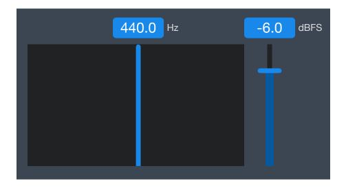
The Oscillator Frequency can go from 10 Hz to 20,480 Hz spanning the entire audio range. We extended the low frequency limit from the traditional 20 Hz down an extra octave to 10 Hz. This is great for testing subwoofers!
