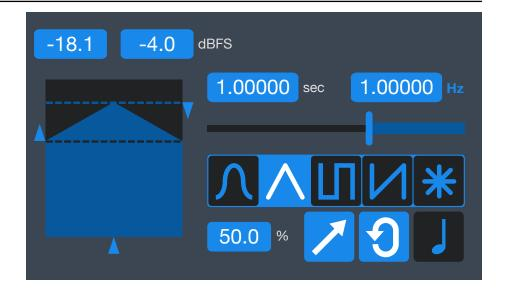
Similar to Frequency Sweep Mode, we have a control for setting the Sweep Period in seconds. This is how long it will take for the level to change from its minimum setting to its maximum setting or vice versa. Alternatively, you can set the Sweep Rate in Hertz.
