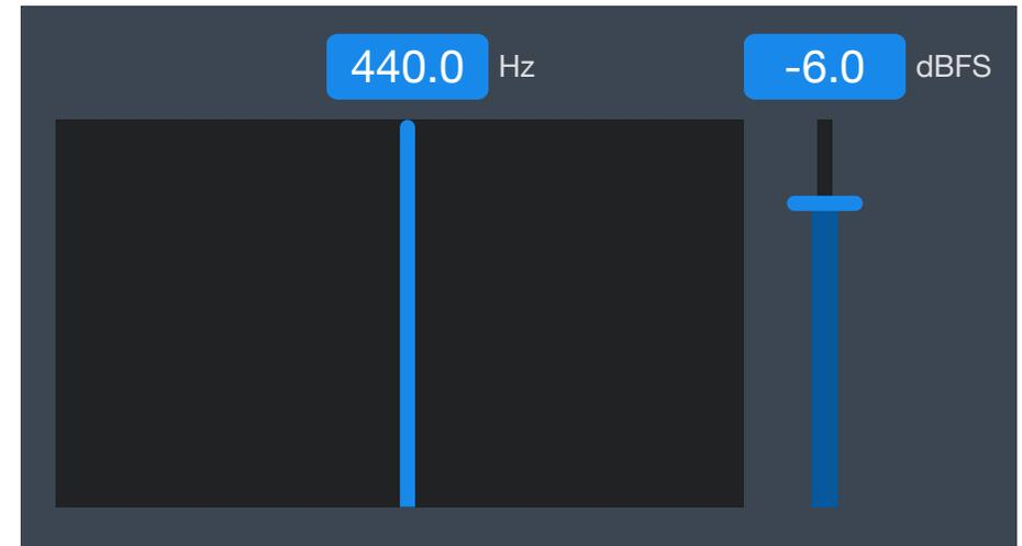
The Oscillator Frequency can go from 10 Hz to 20,480 Hz spanning the entire audio range. We extended the low frequency limit from the traditional 20 Hz down an extra octave to 10 Hz. This is great for testing subwoofers!
